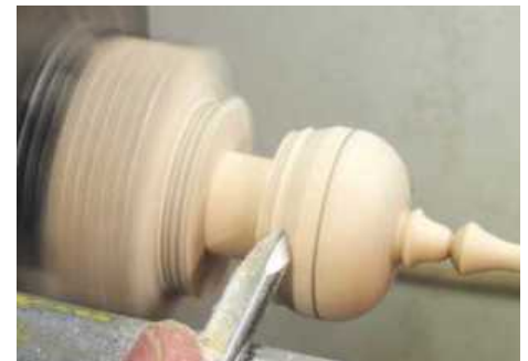
▲ Pic.6 The bulbous bit at the top of the icicle is a simple bead. The pencil line in the centre is a guide for me to turn the bead evenly – the spindle gouge is perfect for this, but use the skew if you are confident in doing so
